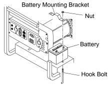
Figure 12 - Battery Hold-Down System (Model RGH7500AIE Shown)
